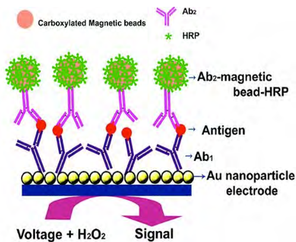
Figure 1. Scheme of the gold nanoparticles immunosensor. The detection step involves immersing the sensor into buffer containing mediator, applying voltage, and injecting H 2 O 2 .
