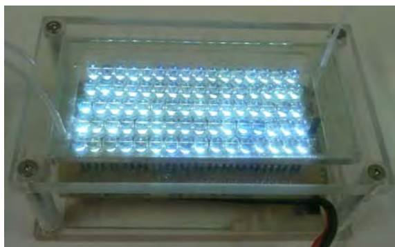
Figure 1 - Photochemical microreactor with white LED illumination
