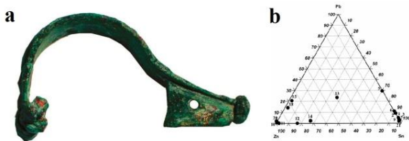
Fig.4. Sample 11 (a) and ternary diagram Sn-Pb-Zn (b).
