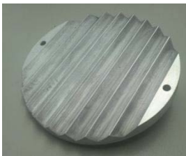
Fig. 5: Faraday cup collector 90^\circ .
