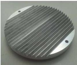
Fig. 6: Faraday cup collector 45^\circ .
