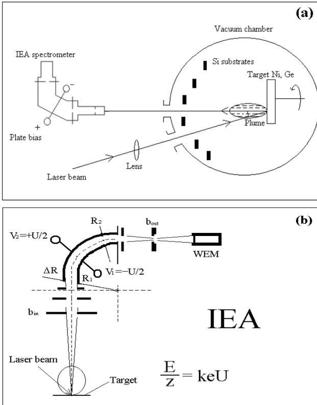
Fig. 1. (a) Scheme of the experimental setup. (b) Scheme of the Ion Energy Analyzer (IEA).
