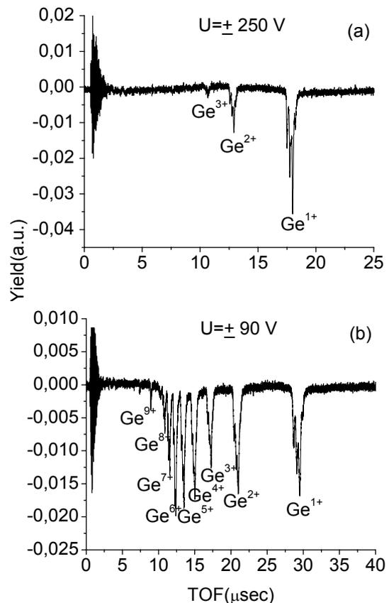
Fig. 2. Ge ion yield vs. TOF of emitted ions analyzed with a plate bias of  $\pm 250 \text{ V}$  (a) and  $\pm 90 \text{ V}$  (b).
