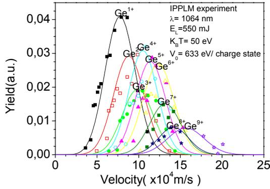
Fig. 3. Ion velocity distribution obtained at IPPLM of Warsaw
