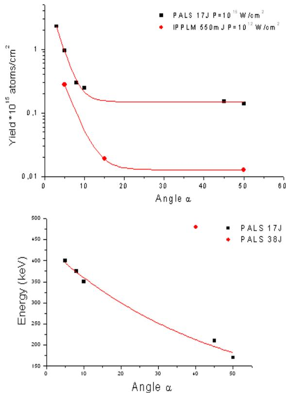
Fig. 5. Ge yield vs. angle for IPPLM and PALS experiment (a) and Ge ion energy vs. angle for PALS experiment at two laser energies.
