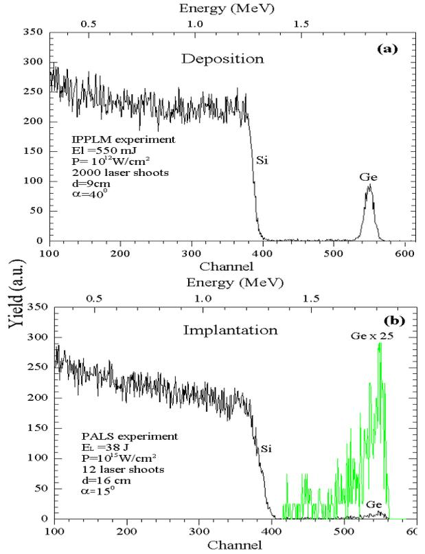
Fig. 4. RBS spectrum of deposited Ge film at IPPLM (a); RBS spectrum of implanted Ge ions at PALS (b).
