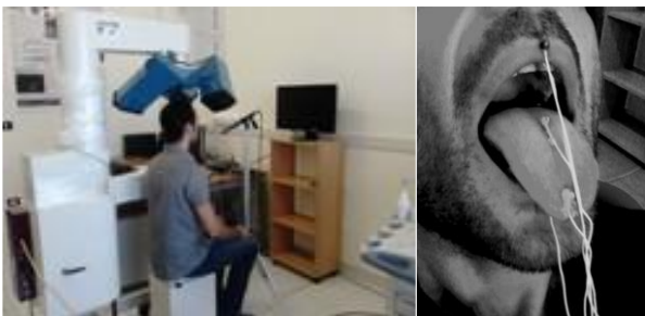
Figure 2. Speech recording with AG501 (left) and sensors glued on the subject's tongue and lips (right)
